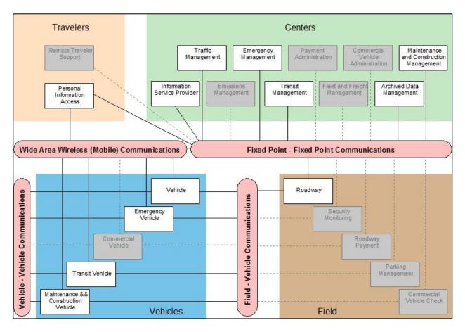
This shows the four essential elements – Travelers, Centers, Vehicles, and the Field – all of which have various subsystems that were identified during the creation of the architecture. The diagram represents how the various elements interact with each other to achieve the desired outcome(s). For example: Roadway information from a Traffic Management Center can be distributed through field-vehicle communications to vehicles.
