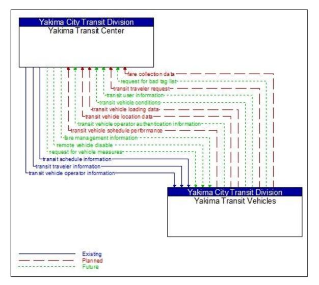
The Flow diagram shows the various existing, planned and future elements that have been identified between systems. As with the Interconnects diagram, the Flow diagram can include additional systems – but can get confusing quickly if too many are selected.
